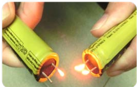
◆ 短路实验 Short circuit test
