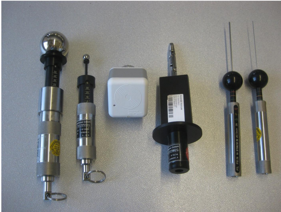
Picture 1: Sample with access probes
